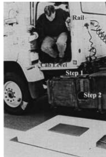
Figure 1- Forceplate setup for exiting from conventional tractor cabin [2].
