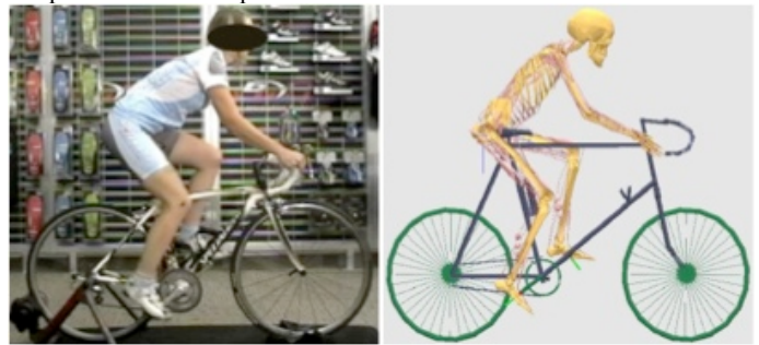
Figure 1. Participant in cycling fixture and corresponding scaled musculoskeletal model (the bicycle frame is un-scaled and used only for visualization purposes).
