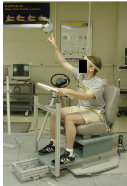
Figure 1. Participant in the test facility, showing rotating seat, computer-controlled target-positioning apparatus, and motion capture hardware.
