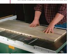
You could use a router and a straight bit to make this cut as long as you had a reliable way of guiding the router (such as an edge guide). I find a table saw is much faster for this operation.
