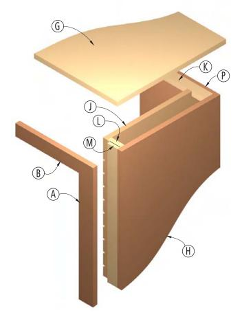
Mark the base cutouts on the sides, front and plywood back of the case using the diagrams as a guide. Use a jigsaw to make these cuts and clean up your work with sandpaper.
