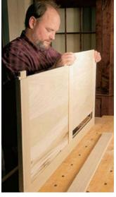
You can see the haunch on the tenons on the rail closest to the camera. When it comes to fitting your panels, remember to work tight in summer and loose in winter. Panels of this size will shrink and contract noticeably.
