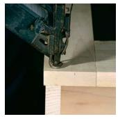
I'm not perfect, and neither are you. If your face frame is exactly the width of your case, it's going to be difficult to fasten it square. Make life easier by ripping your stiles <sup>1/</sup>16" oversize in width. After you nail and glue the face frame to the case, use a flush-trimming bit in your router to trim the face frame flush with the side of the cabinet's case.
