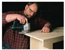
In addition to cutting this detail on the sides and front (above), I also cut it on the bottom of the plywood back, which gives it a finished look when the cabinet is viewed from down low or from a distance.
