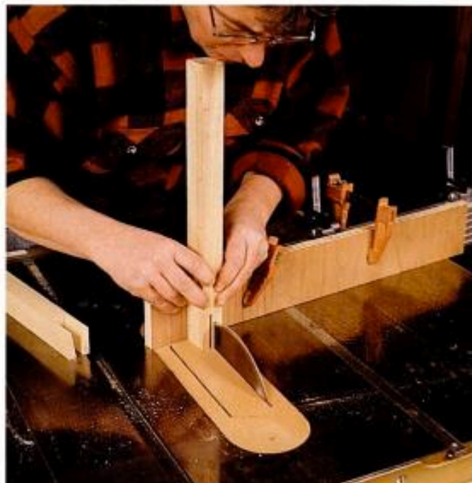
Pins second. With the miter gauge angled at 8°, Staples saws the dovetail socket in the suspension arm by holding the work against a high fence attached to the miter gauge.
