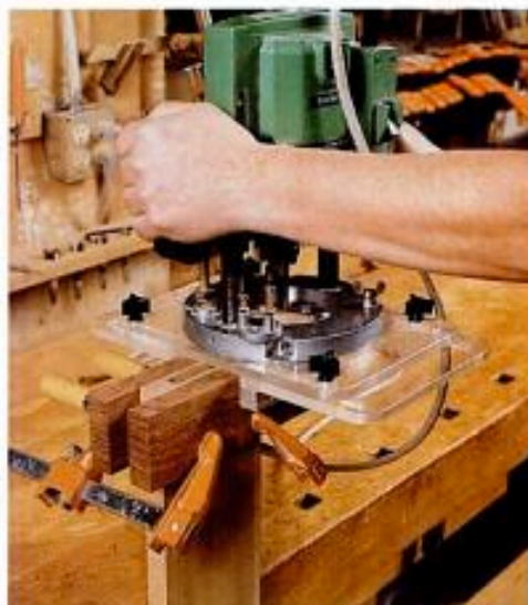
Plunge rout the mortise. Staples uses a 1/2 -in. upcut spiral bit and a pair of fences attached to the router baseplate to rout the mortise in the end of the stretcher.
