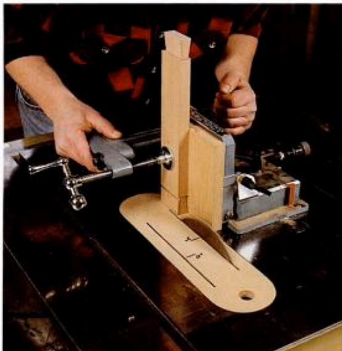
Tails first. The author angles the blade to 8° and clamps the pivot-block stock in a Delta tenoning jig to saw the sliding dovetails.
